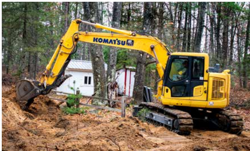
Curtis Excavating operator Andy Curtis moves dirt with a Komatsu PC138USLC tight tail swing excavator.
